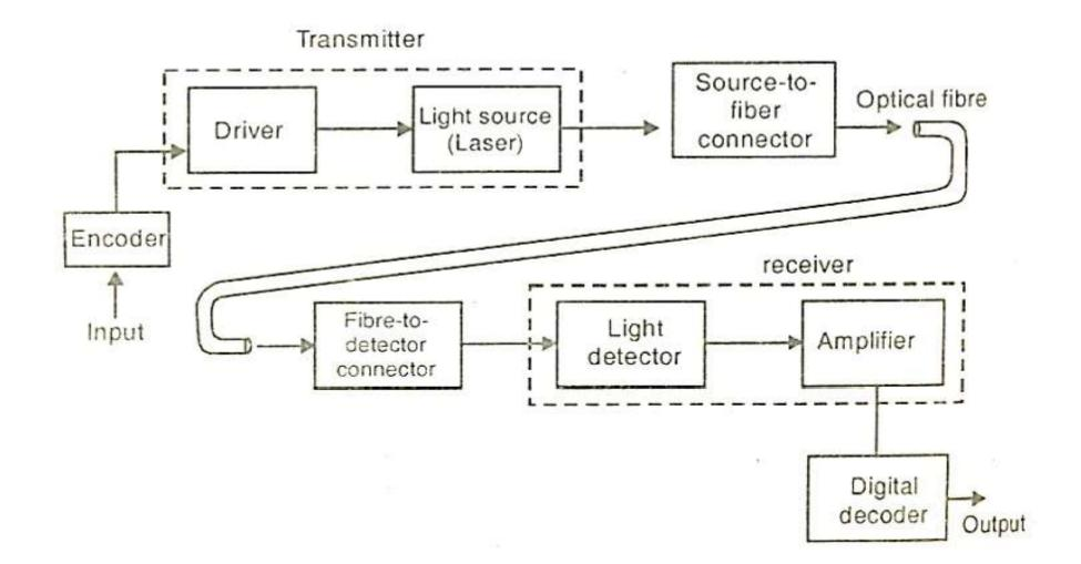
The major components of an optical fiber communication system are
