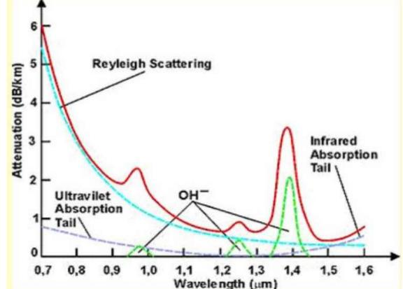
Ion resonance absorption is caused by  $OH^-$  ions in the materials. The source of the  $OH^-$  ions in water molecules that have been trapped in the glass during the manufacturing process. Iron, copper and chromium molecules also cause ion absorption
